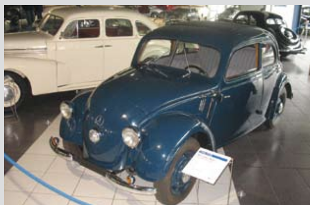
Mercedes-Benz 170 H (W 28) Limousine (1936-1939) Farmotor, 4 henger, soros, SV, 1697 cm 3 , 38 LE
