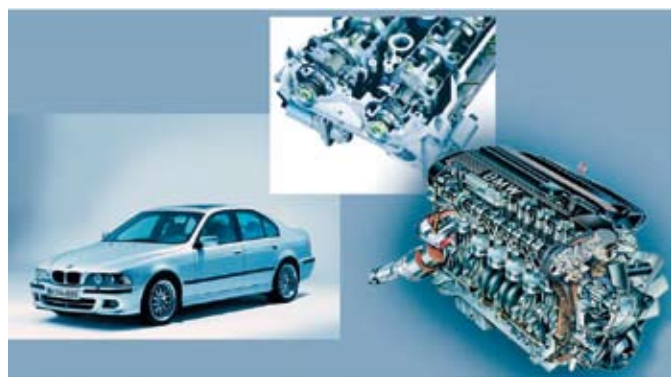
1 1997 – BMW 528i, motor: M52B28TU, 4 szelep, DOHC, bi-VANOS (Doppel-VANOS)
