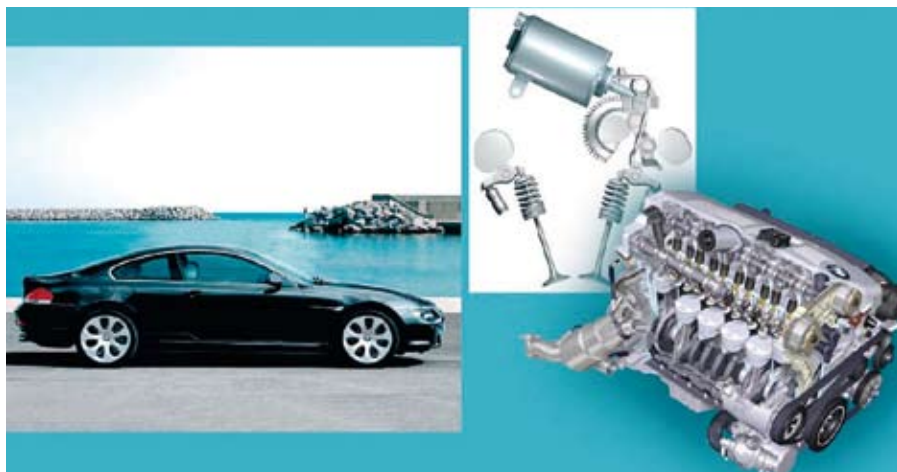
3 2005 – BMW 630i, motor N52B30OL, 4 szelep, DOHC, bi-VANOS, VALVETRONIC II
