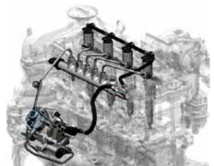
5 A common rail rendszer elemei
